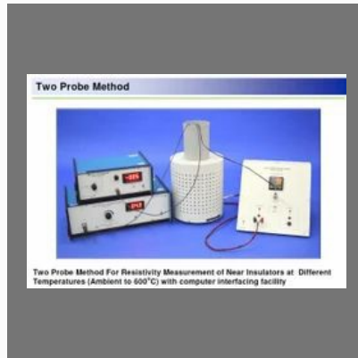
High Temperature Two Probe Set Up
